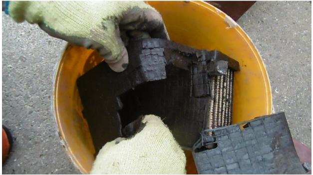
Note that there is hardly any shedded plate material in the reservoir below the cells. It's not shedded material shorting the underside of the cells, as it
