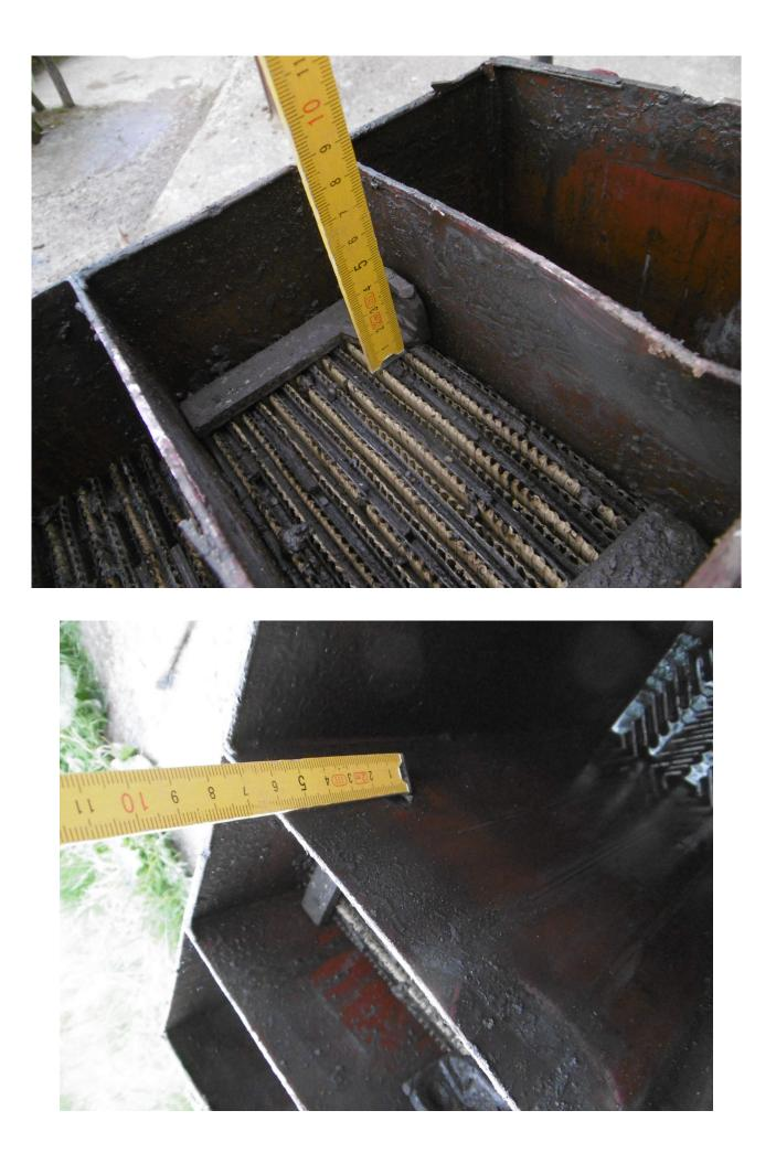
The anode plates disintigrate because the connecting frame is too weak. That explains why it seems impossible to balance the cells, some parts of the plates are simply not connected. The silvery looking cathodes are in a reasonable state, the reddish anodes are just falling apart, with the anode frames partially fractured.
