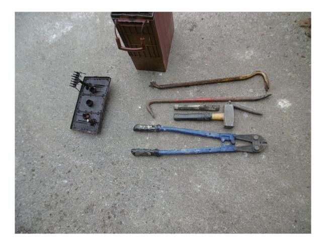
Before prising off the lid, seperating the cells and sliding out one set of plates for closer inspection the battery was carefully drained. Then the plates and casing were repeatedly washed out with a warm bicarbonate solution. This is dangerous - do not try this at home. If you must: protect eyes and skin. You're clothes will likely be for the bin afterwards.
