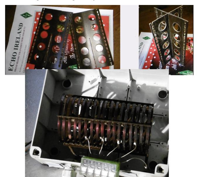
Images above: A homebrew tapped 12 microHenry coil, relais switched taps are at 2, 3, 5, 8 and 12 microhenry. This coil loads a 160m Half Quad, covering the full band. Made with flat 6x3 mm flat wire to keep parasitic inter-turn capacity low, on a pertinax coil former.
